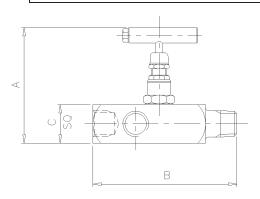
The 'GM1' Type Gauge Multiport Needle Valve is designed for safe and reliable isolation, giving bubble tight shut off, with non-rotating & anti-galling tip and dynamic self-adjusting spindle seal to give long service life in a variety of applications. The valve has three outlet connections for flexible instrument hook up plus the ability to calibrate the instrument in-situ.
